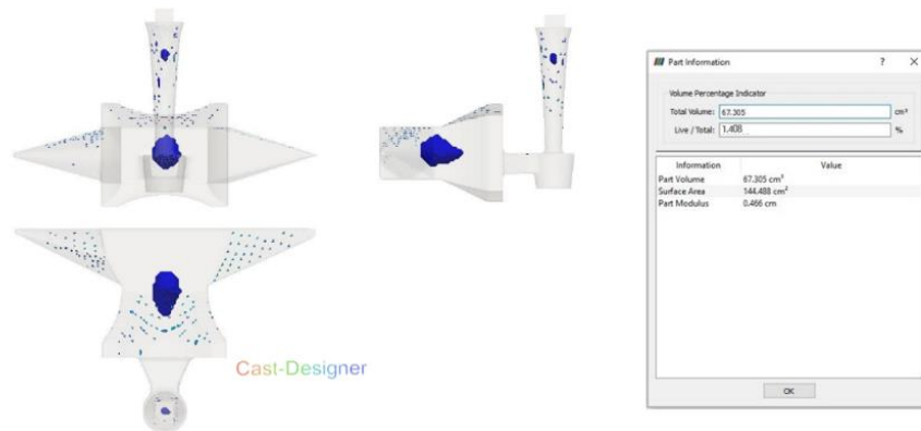
Figure 10 Shrinkage Porosity Simulation for Trapezoidal Mold Sample 22.
